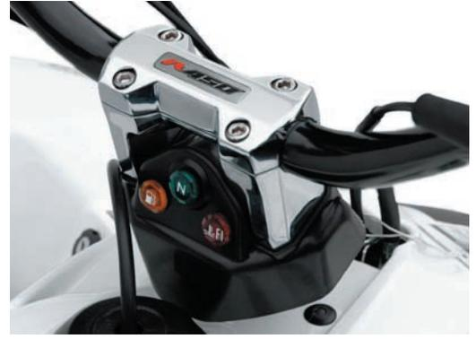
There is a bend in the aluminum bar clamp. It should face toward the front of the quad. Backwards installation will cause the control cables to not be long enough during cornering.
